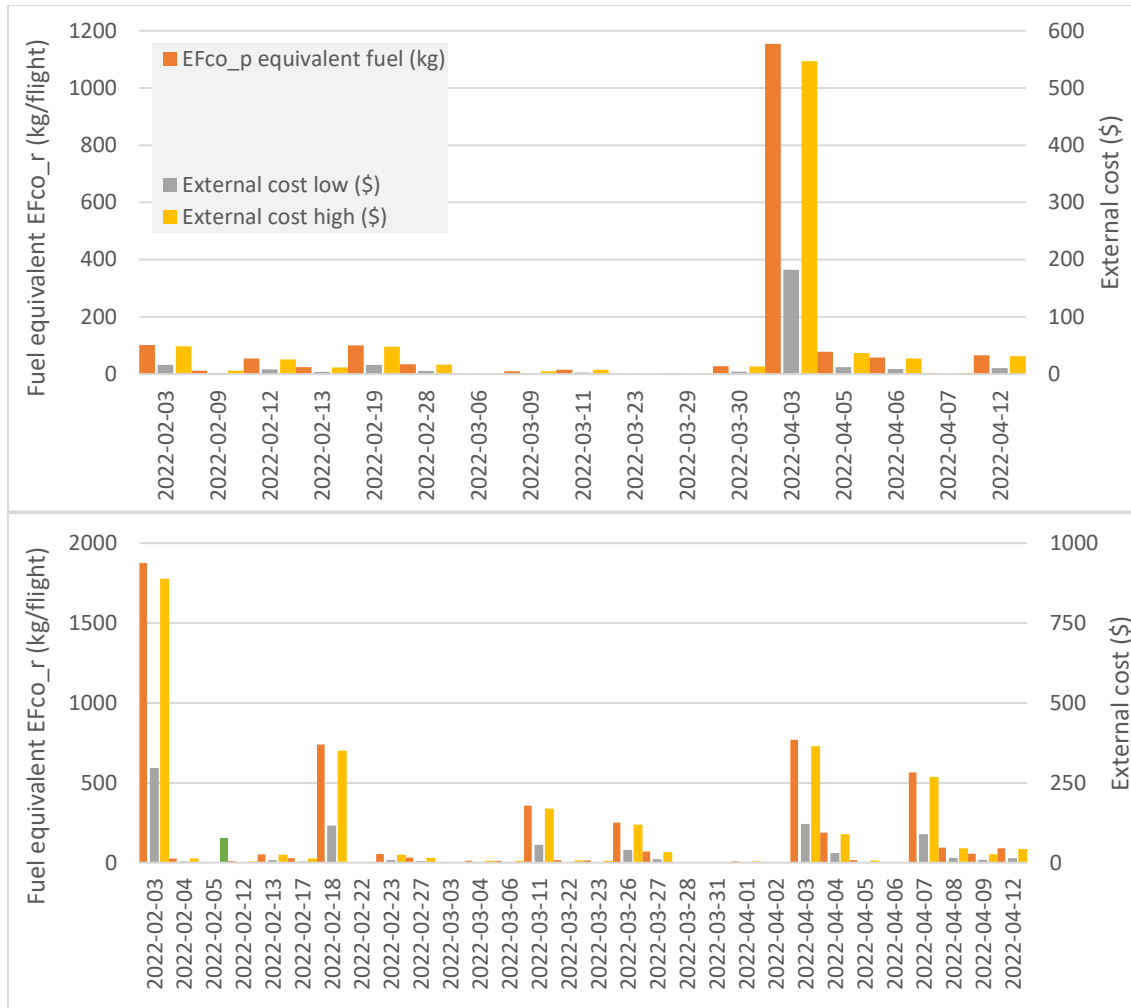
Figure 5.8. Kg of fuel with CO 2 emissions equivalent to EF co_r (on 20-years horizon) for each flight with positive energy forcing on route HEL-AMS (upper panel) and ARN-KRN (lower panel) and the corresponding external costs of flights (assuming external cost of 1t CO 2 eq = 1000 $).
