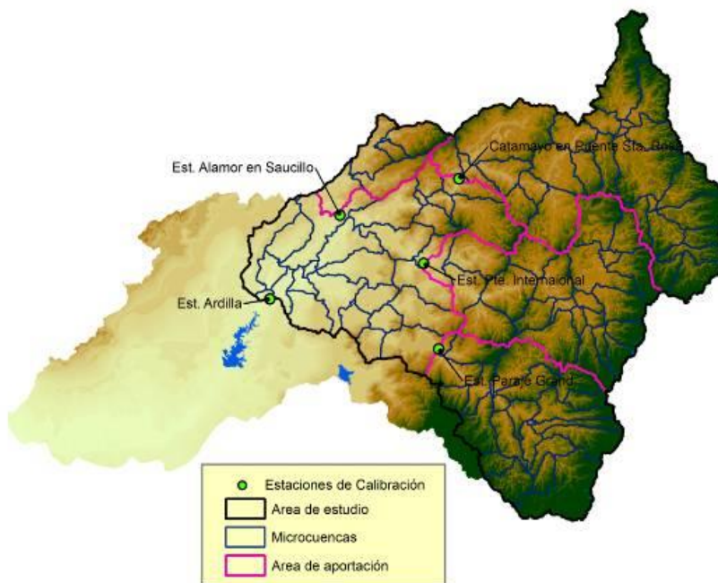
Figure 40. Location of the five measurement stations of used streamflows in the calibration of SWAT.
