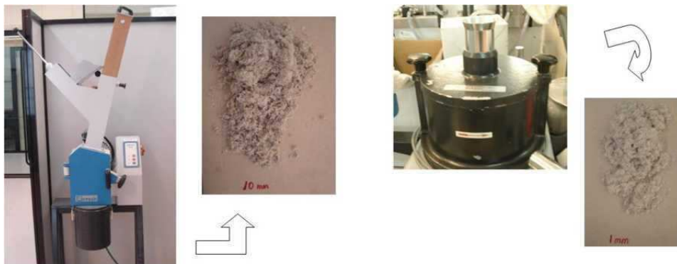
Figure 10. Equipment used for material milling and different sizes obtained for recyclability tests
