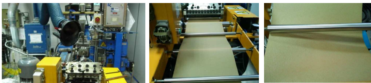
Figure 7. Processing of recycled material by ONE STEP process in compounding machine
