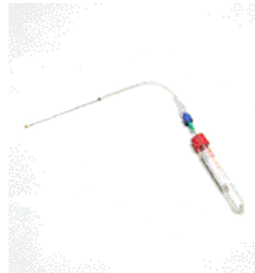
Figure 8. Rhizon sampler with vacuum flask (Eijkelkamp, 2004).
