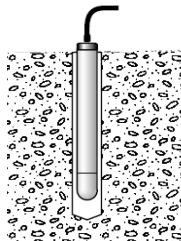
Figure 7. Vacuum lysimeter (Soilmoisture Corp, 2004).
