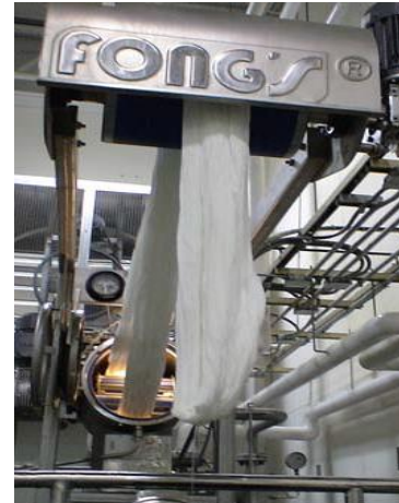
Figure 1. Low-Liquor Jet Dyeing machine (Cotton Inc., 2009)
