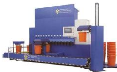
Figure 2. Automatic Dye and Chemical Dispensing (Cotton Inc., 2009)
